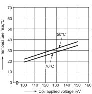
4. Ambient temperature characteristics Tested sample: PQ1a-24V Contact carrying current: 5 A
