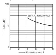
5. Electrical life test (10 A 277 V AC, resistive load) Sample: LKP1aF-12V, 6 pcs. Operation frequency: 20 times/min. (ON/OFF = 1.5s: 1.5s) Ambient temperature: 20°C 68°F
