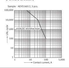
4. Switching and cut-off life curve (Forward direction)
