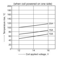
1.-(5) Coil temperature rise (at room temperature)
