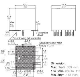
1 to 3mm .039 to .118 inch:  $\pm 0.2 \pm .008$ Min. 3mm .118 inch:  $\pm 0.3 \pm .012$
