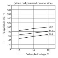
1.-(3) Coil temperature rise (at room temperature)
