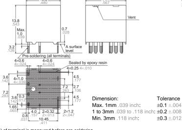
Dimensions (thickness and width) of terminal is measured before pre-soldering. Intervals between terminals is measured at A surface level.
