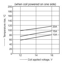
1.-(2) Coil temperature rise (at 85°C 185°F) Sample: ACJ1212, 3pcs Measured portion: Inside the coil Contact carrying current: 10A, 15A, 20A Ambient temperature: 85°C 185°F
