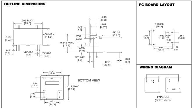
Dimensions in inch with millimeters in brackets below. Tolerance:±.010"
